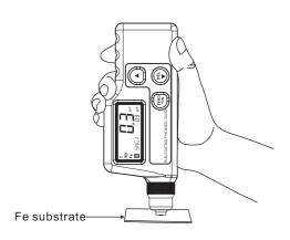
b. Do not lift the sensor tip and press the ZERO/ON key, the buzzer sounds indicates Zero point calibration is completed. LCD displayed like the following picture at this time:
