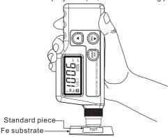
c. Do not lift the sensor tip and press the UP and DOWN key to correct the reading, after these the calibration is completed, the instrument is ready to process. LCD displayed like the following picture at this time:
