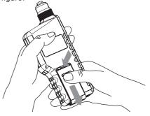
2). Insert the 9V battery into battery compartment, note the battery polarity, and then close the battery door, as shown in the following figure:
